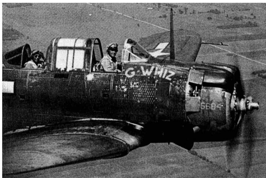
FIGURE 3. The A-24, Douglas Dauntless Dive Bomber, loaned to the Mayo Aeromedical Unit and specially instrumented by Dr. E. H. Lambert for comparison of the effects of +G , acceleration in a healthy man during exposures when acting as subjects on the Mayo Human Centrifuge, when riding as passengers, and when piloting this aircraft, 1945. (Reproduced from Wood, E. H., Ann. Biomed. Eng. , 6, 250, 1978. With permission.)
